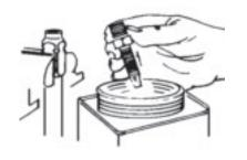
2. Oil inside of hose and the tapered nipple thread areas liberally with oil. Do not oil hose cover. Apply anti-seize to all thread areas.
