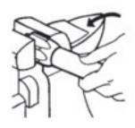
1. Place socket in vice and screw in hose counter-clockwise until hose bottoms. Back hose out 1/2 turn.
